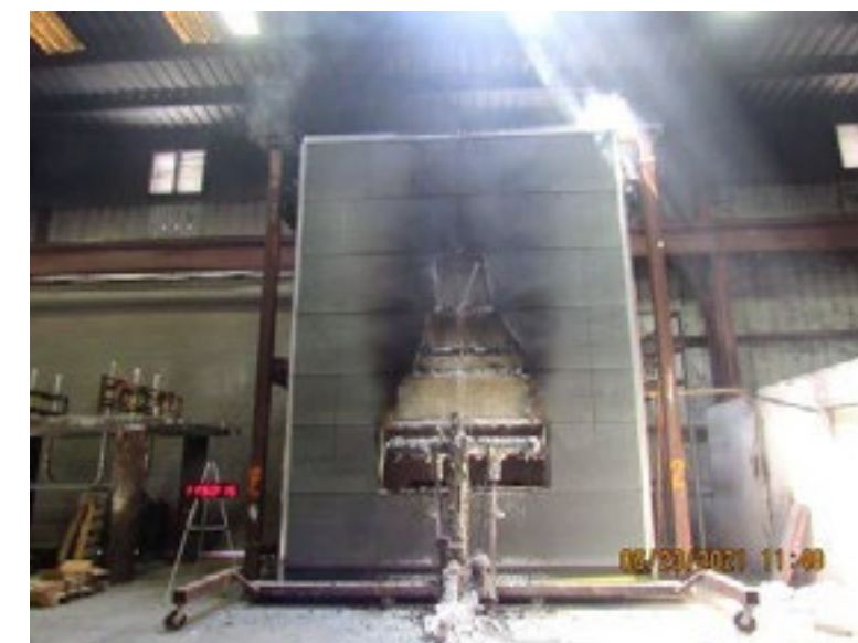
Photo No. 2 4 mm Alfred FR Zinc Composite Wall assembly after test.
