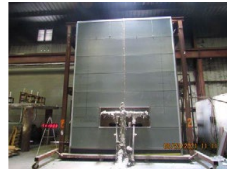
Photo No. 1 4 mm Alfred FR Zinc Composite Panels Wall Assembly Before Test.
