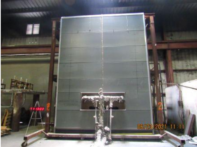
Photo No. 1 4 mm Alfrex FR Zinc Composite Panels Wall Assembly Before Test.
