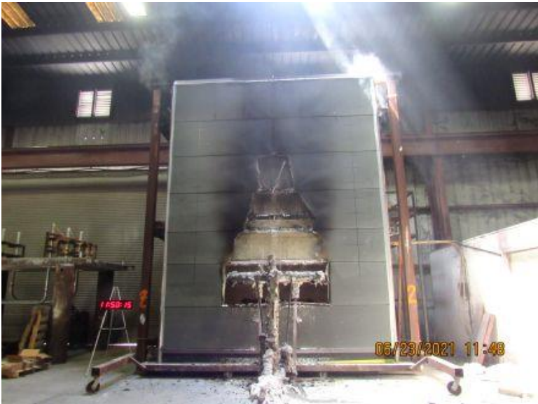
Photo No. 2 4 mm Alfrex FR Zinc Composite Wall assembly after test.
