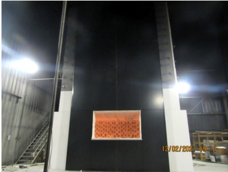
Photo No. 1 4 mm Alfred aluminum composite panel Wall assembly Start of Test.
